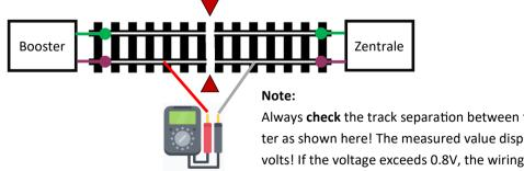
Always check the track separation between the control centre and booster as shown here! The measured value displayed must not exceed 0.8 volts! If the voltage exceeds 0.8V, the wiring and the voltage setting on
