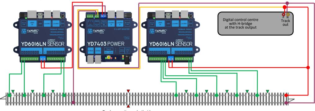
Track separation on both sides between control centre and booster
