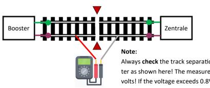
Always **check** the track separation between the control centre and booster as shown here! The measured value displayed must not exceed 0.8 volts! If the voltage exceeds 0.8V, the wiring and the voltage setting on the power supply unit must be checked.
