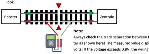
Always check the track separation between the control centre and booster as shown here! The measured value displayed must not exceed 0.8 volts! If the voltage exceeds 0.8V, the wiring and the voltage setting on
