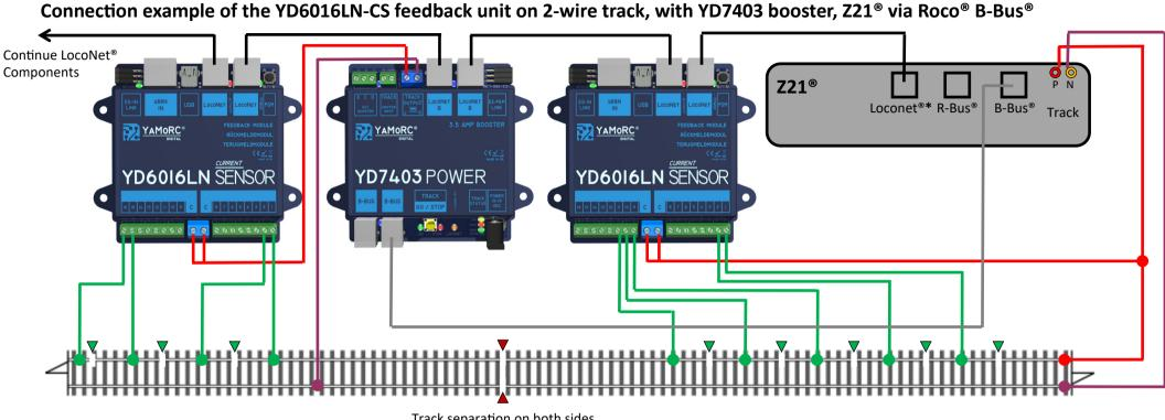
Track separation on both sides between control centre and booster
